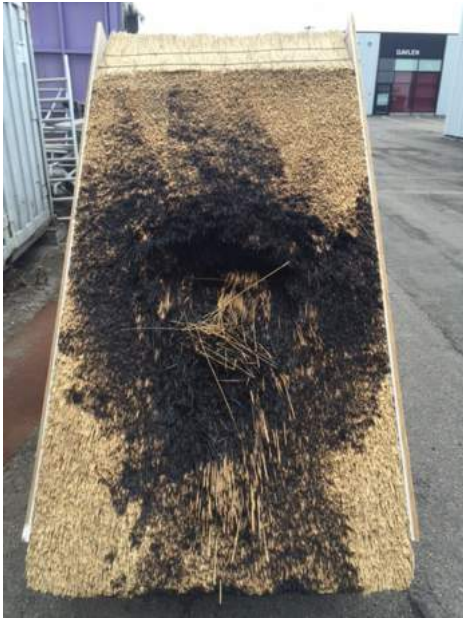
Photo 10: Roof model 1 (no cavity).
