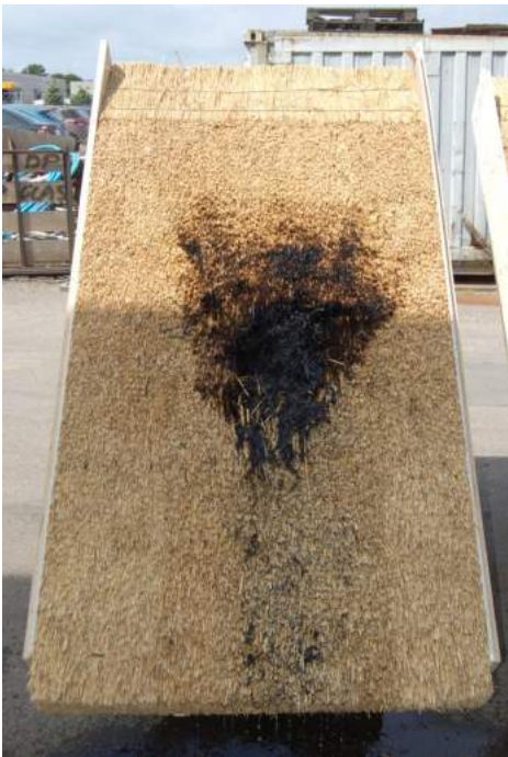
Photo 12: Roof model 3 (60 mm cavity and Sepatec).
