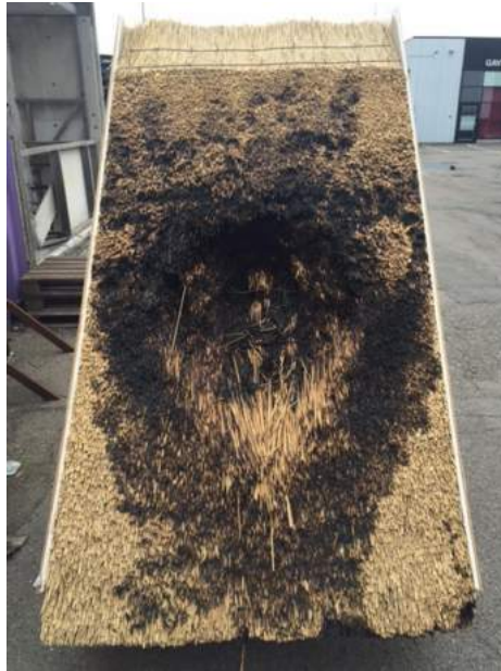
Photo 11: Roof model 2 (30 mm cavity and Sepatec).
