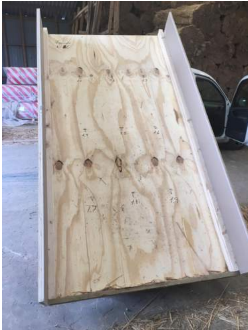
Photo 1: Underlying class EI 30 building element of a material of at least class D-s2,d2 (two layers of 18 mm plywood).
