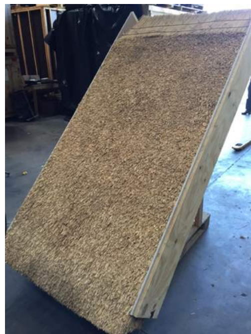
Photo 4: Finished roof model.
