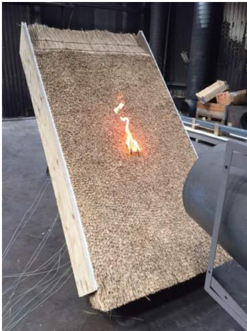
Photo 6: Immediately after exposure to the ignition source.
