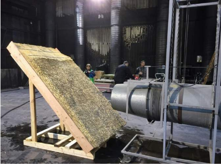
Photo 5: Test setup of roof model and wind turbine.
