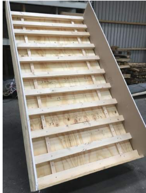
Photo 2: Construction of batten layers (roof models 2 and 3) with cavity facing the underlying class EI 30 building element.
